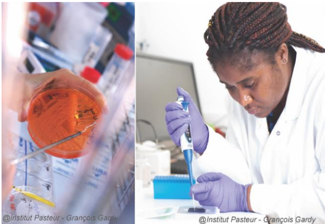
Figure 14. MALDI-TOF experiments at the CRBIP. Sampling from Shigella colonies; preparation plate for MALDI-TOF analysis.
